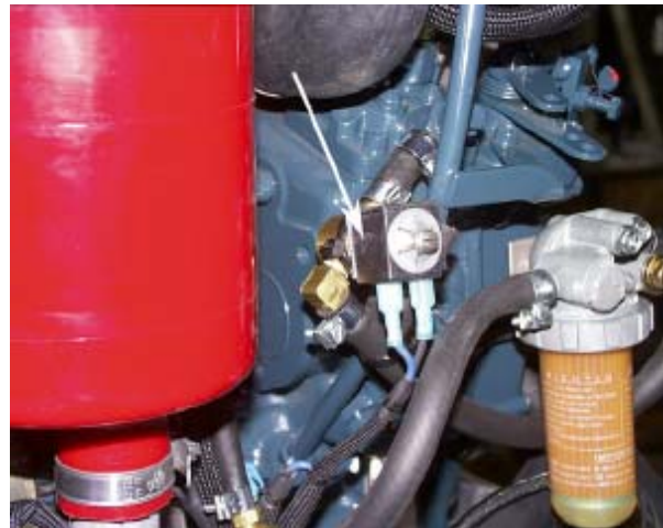
Unplug one of the fuel solenoid wires from the unit harness.
