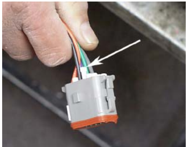
Remove the cavity plug. Save it for replacement
