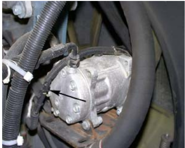
Single-wire harness plug on a truck compressor.
