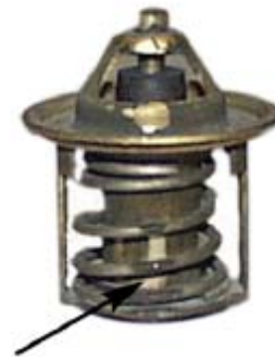
Close-up of a stuck thermostat
