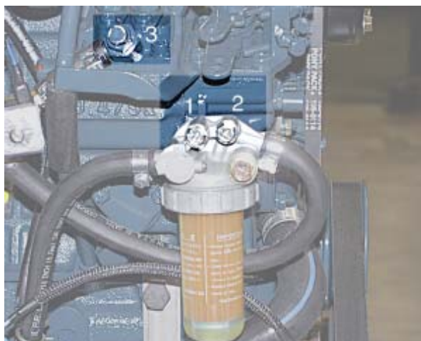
Three purging screws: (1) and (2) on the aluminum filter body and (3) on the injector pump.
