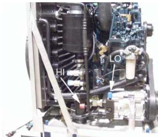
Hi and lo pressure service ports for hooking a set of refrigerant gauges to the Pony Pack.
