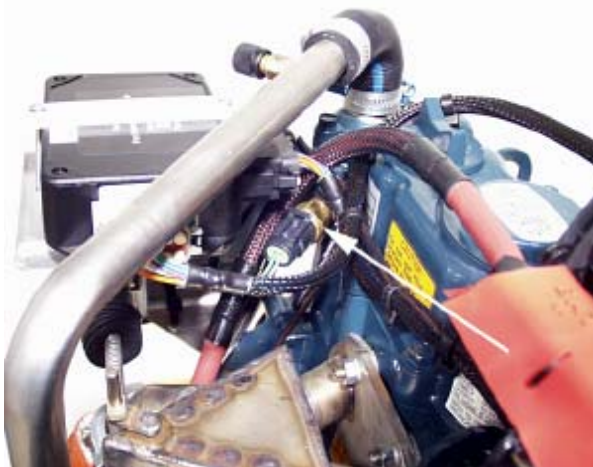
Coolant fluid sensor in the Kubota thermostat housing
