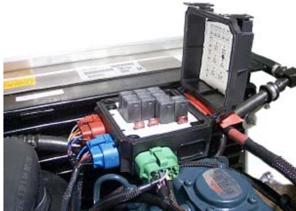
Pony Pack load center with the lid open to show the fuses and relays.
