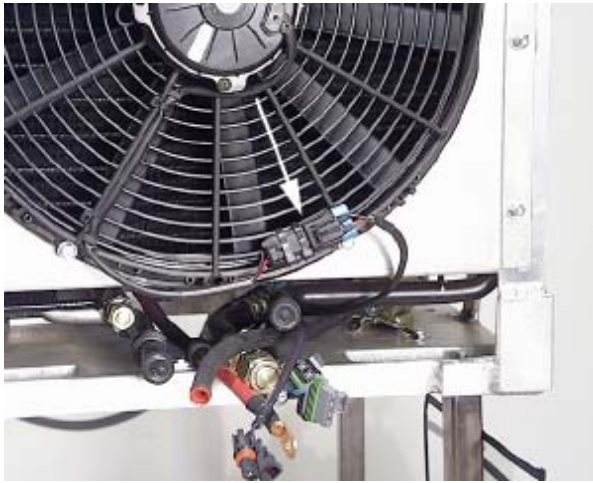
Harness fan connection behind the unit
