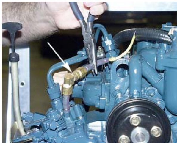
Squeeze the hose between the fuel return check valve and the injector pump
