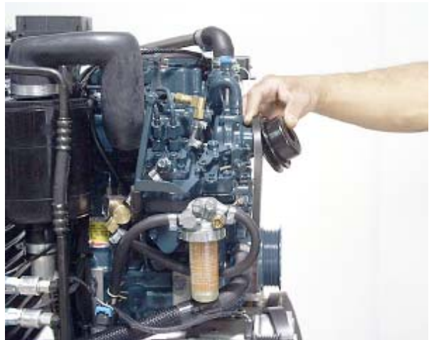
Angle the pulley onto and over the hub.
