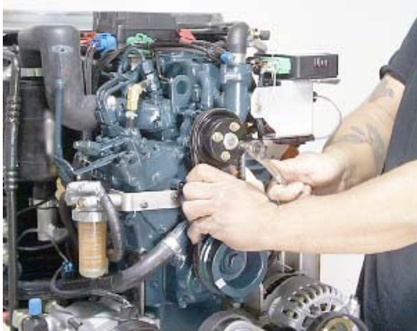
Remove the four water pump pulley bolts. The belt squeeze method is used to keep the pulley from turning.
