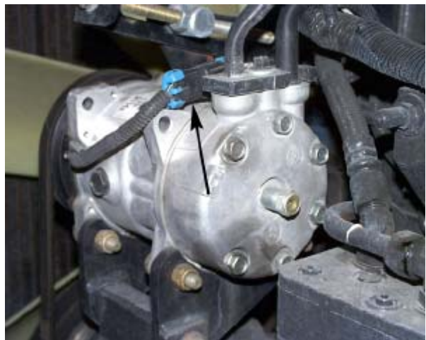
Two-wire harness plug on a truck compressor
