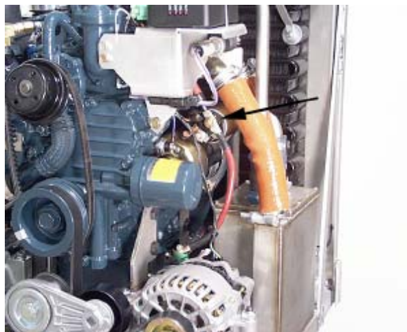
Cable connections at the stud on top of the alternator.
