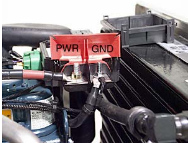
Load center power and ground studs: The Power Stud is the larger of the two.
