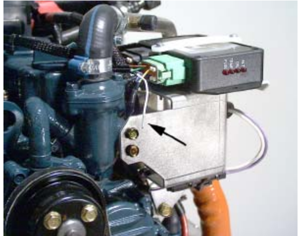
The reset wire is a short white wire in the green module connector.
