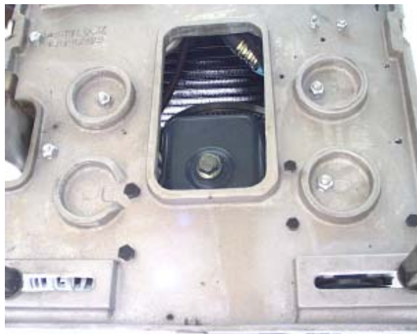
Remove the drain plug with a 22 mm socket.
