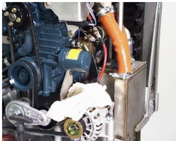
Unscrew the filter cartridge. Use the bottom one inch of an oil or antifreeze jug to catch any oil that spills out of the filter and engine. Use rags to keep oil out of the alternator.
