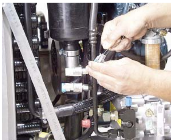
Crossing the fan switch plug in the harness to test the fan switch circuit.
