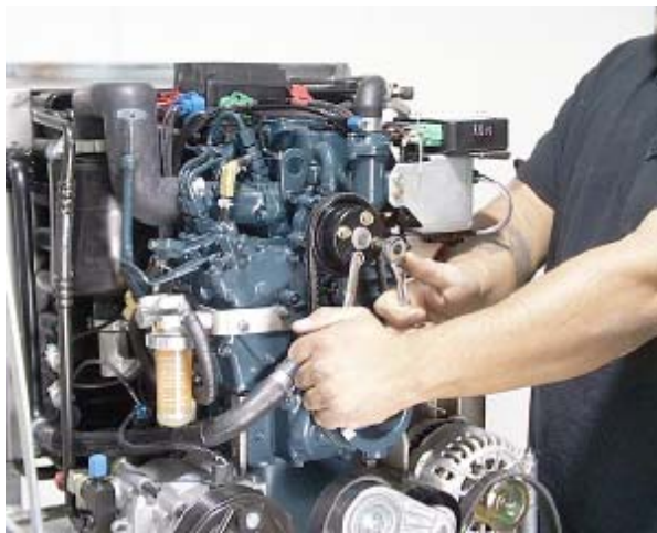
Remove the four water pump pulley bolts. The screwdriver method is used to keep the pulley from turning.
