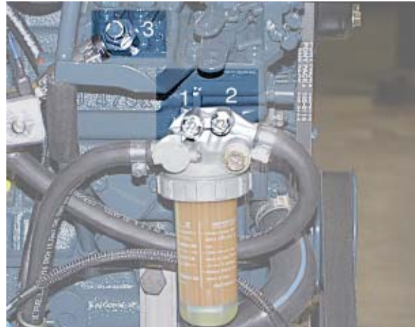
Three purging screws: (1) and (2) on the aluminum filter body and (3) on the injector pump.
