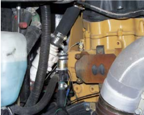
Cab heat pump, properly secured with a cushion clamp.
