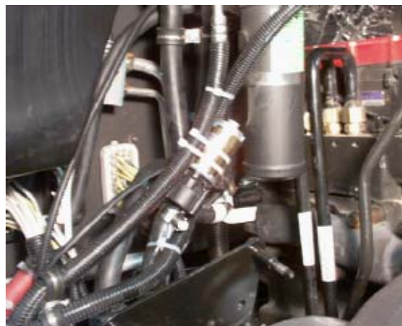
Cab heat pump, properly secured.
