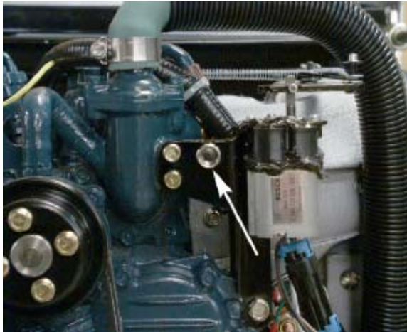
Service button on a model 105 Pony Pack. On older models, this switch is located on the module.
