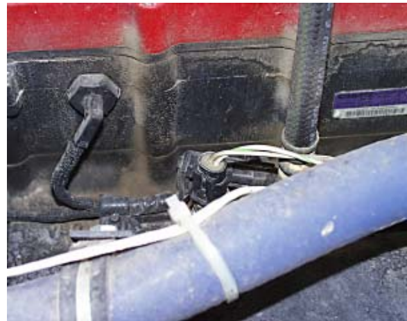
Thermistor installed in truck engine block.
