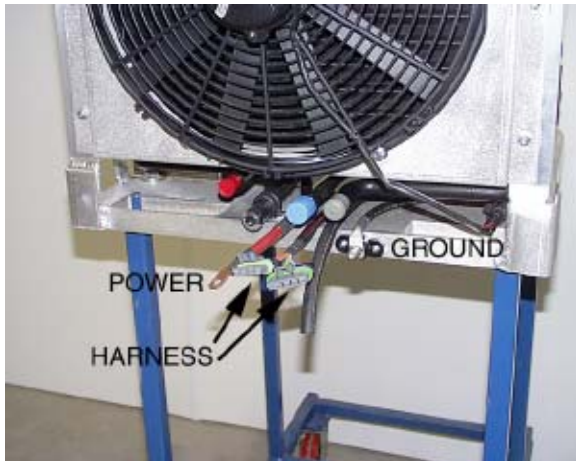
Harness connectors and ground wire behind the Pony Pack
