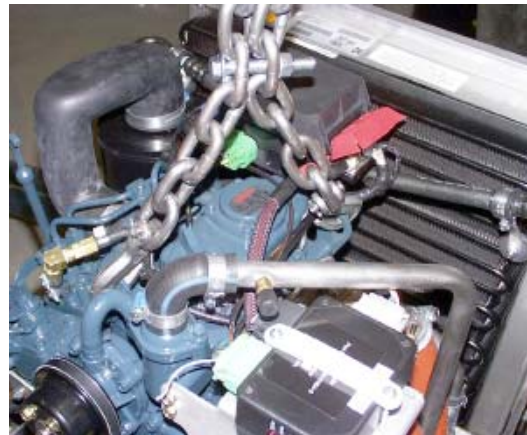
Install a chain hoist to the lifting loops as shown. Notice the bolt to keep the chain off of the load center.
