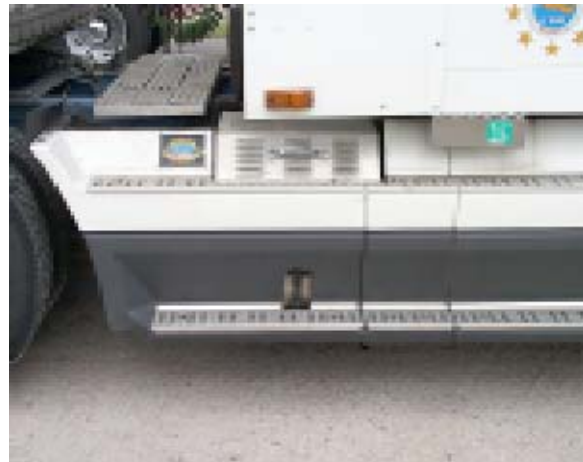
Mounted on a truck with fairings. The Pony Pack cover can be removed without removing the fairing. However, some maintenance and repair procedures would require fairing removal.
