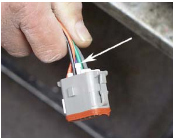
Remove the cavity plug. Save it for replacement.
