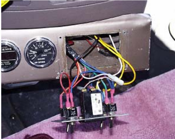
Control panel hanging out of hole in dash with the Pony Pack Cab Harness wires attached.
