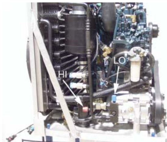
Refrigerant service ports on a model 2006 Pony Pack.
